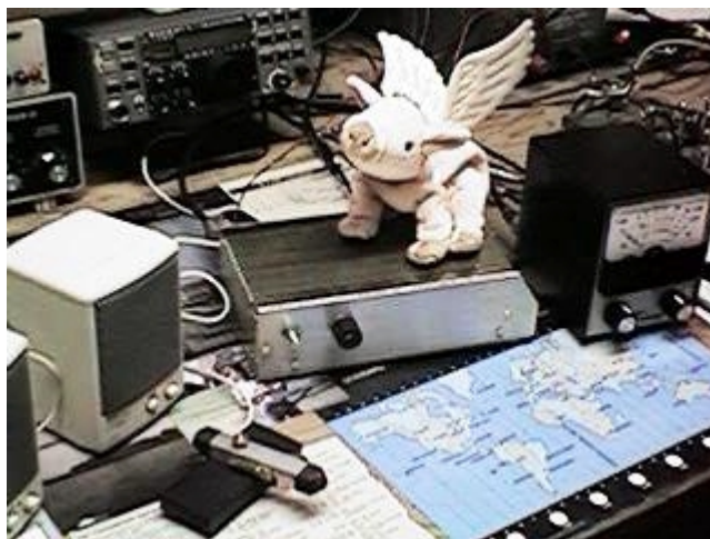
SW40+, speaker, key and WM-2 wattmeter make up complete station. Piggie sits on top of rig to keep QRM out!
