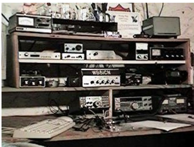
SW40+ sits on the shelf my call sign plaque. This is the QRP side of my operating position...K2 on bottom; TT2 with keyer and tuner on second shelf; SW40+ and my NC40A on the third shelf.
