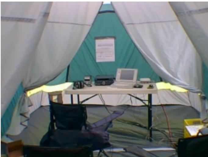
The CW tent, HF2, Fran's TS450 cranked down to 5 watts. The papers taped to the wall are 'cheat sheets' for the TR Logging program.
