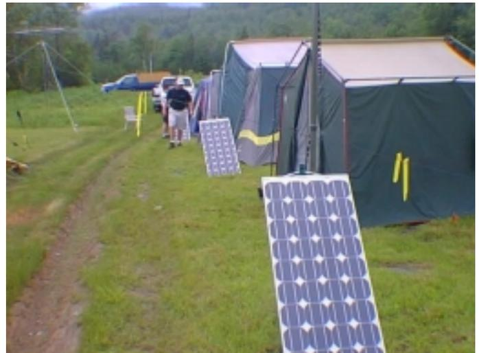
Operating station row, near to far, HF1, HF2, VHF. Each with its own Siemens SP-75 solar panel and deep cycle battery. One continuing comment this weekend was about the blessed absence of the sound of generators. Dick (KG2LN) in background
