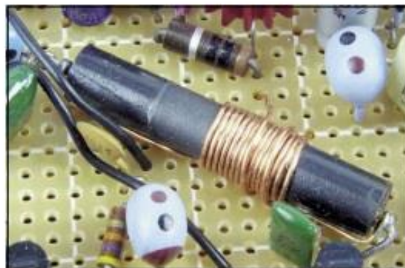
Figure 2—A close-up view of T1, the broadband transformer. I created my version by using a RadioShack 273-102 choke, unwound to 15 turns (10.6 \mu\text{H} ) for the primary. Save the wire! The secondary windings consist of two turns of the removed wire.
