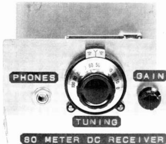
Fig. 49 — Front view of the beginners receiver. The panels are made from double-sided pc board material.
